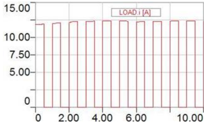
Figure 4. Simulation result-load current
